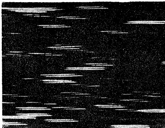
Spectra and inverted spectra of stars observed with an objective prism by Fehrenbach's method. The displacement of corresponding lines permits the star's relative radial velocities to be calculated.
