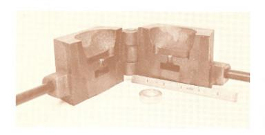
This cast iron book mold for preparing discs of low-melting alloys  $\phi$  1¼" by %" thick permits spectrographers to match their samples to standard discs and so facilitates set-ups and increases accuracy.
