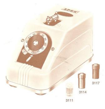
A widely accepted dental tool for triturating amalgams, the standard instrument is particularly useful for mixing and grinding small samples of less than 1 ml.
